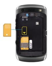
Slide the SIM card into the slot.
